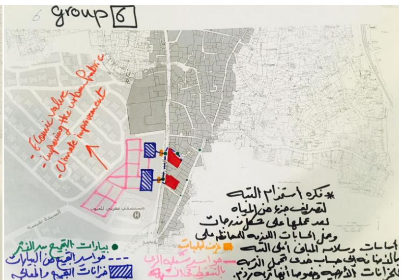
Collect water from historic buildings (Fatima Khatun and al-Ashraf Khalil) by collection pipes then to pump rooms and then to tanks for treatment and to drip irrigation network to cultivate the ridge as steps
