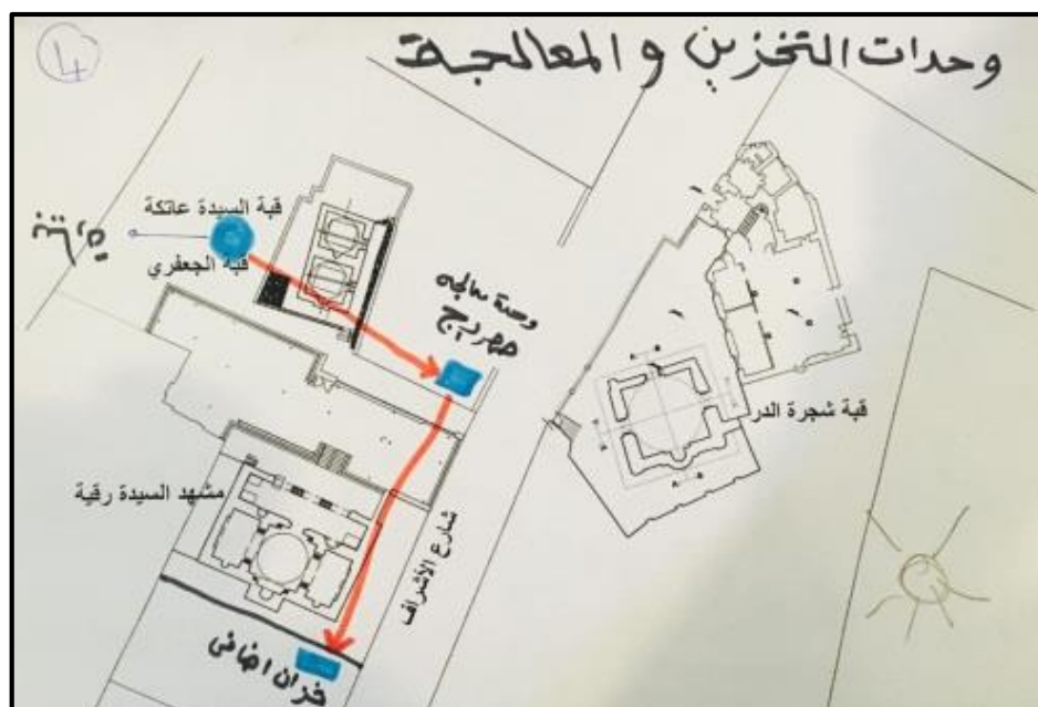
The diagram illustrates proposed storage and treatment units and connections between them
